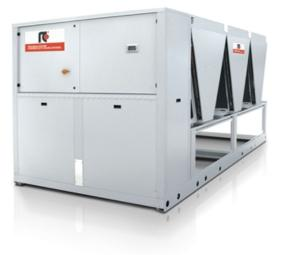
Outdoor unit for the production of chilled water with hermetic rotary Scroll compressors, ozone-friendly refrigerant R410A, axial-flow fans, braze-welded plate-type heat exchanger, micro-channel full-aluminum air coils and thermostatic expansion valve. The range is composed by units equipped with four compressors in tandem configuration on two independent refrigeration circuits.
